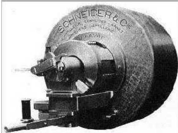
Detail of the head of a barrel of 240 Cannet system
