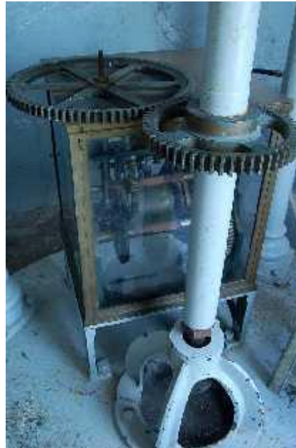
The original turning system designed by the Henry Lepaute Company
