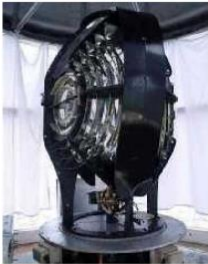
The original turning system designed by the Henry Lepaute Company
