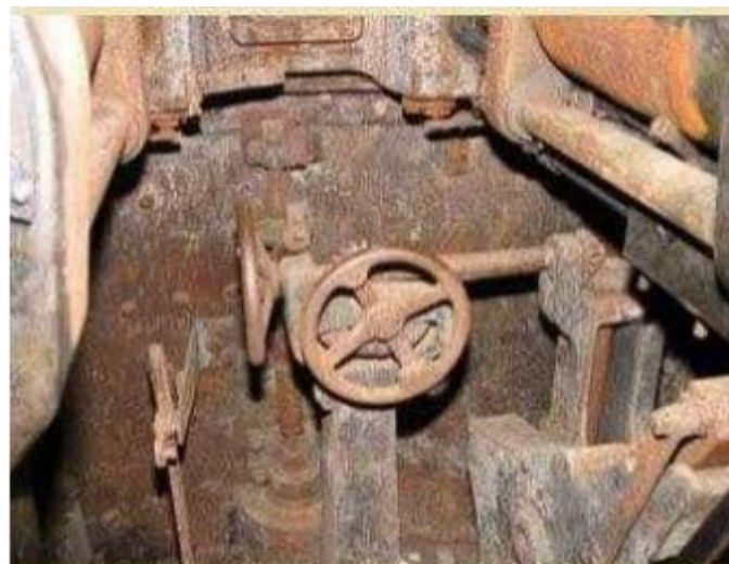
Mechanism of the rotating turret
