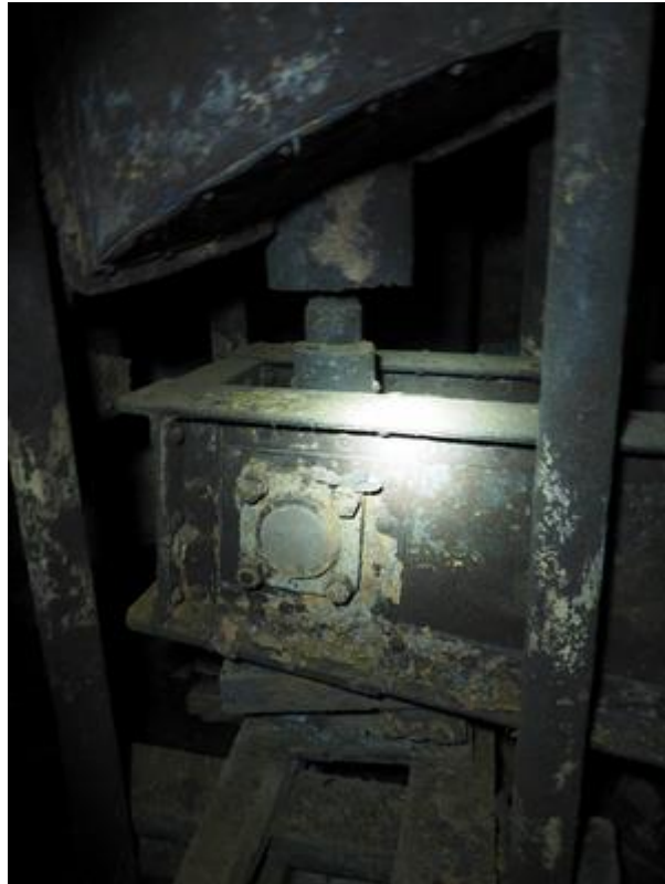
This section raises the cupola column to move up and down in a vertical line by allowing it to swivel when being positioned.
