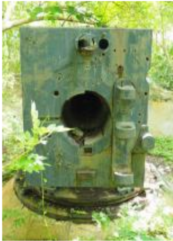
The Barrel with the breech removed on Gun Number 17
