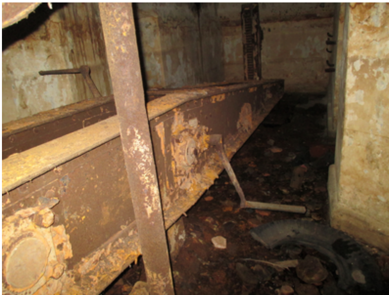
The reverse of the previous, looking back toward the jack. Showing the pivot point and the jacking arms.
